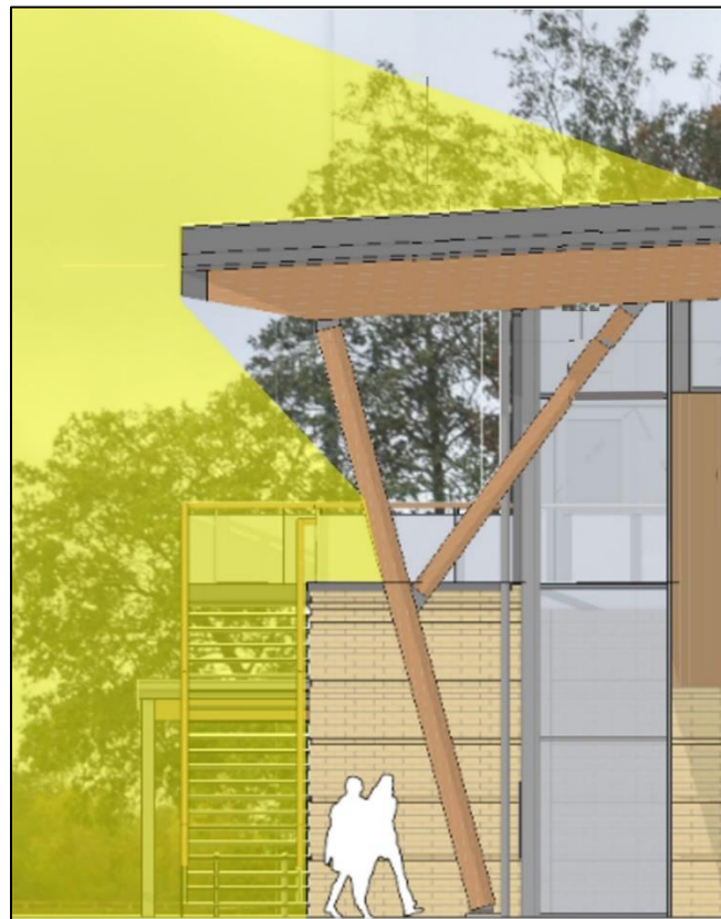
figure 34: DM graphic illustrating the brise soleil effect created by visually elegant roof overhang
